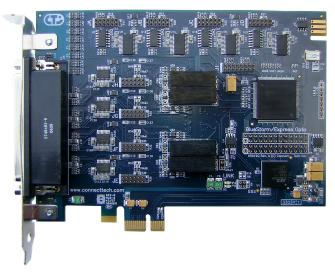
The BlueStorm/Express Opto (1 kV) card demonstrates Connect Tech's commitment to customer satisfaction as it provides a perfect example of a board that was developed to support specific customer requirements. Designed to significantly protect data communications within budgetary restraints, BlueStorm/Express Opto (1 kV) offers multi-strike surge suppression on four ports of eight ports and the added protection of optical isolatation on the remaining four ports.
