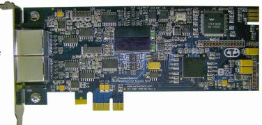
An extension to the BlueStorm/Express product family, the BlueStorm/Express LP Opto offers a low profile solution (standard height bracket available) for your PCI Express applications. Dependability and high speed data transfer rates along with 3kV optical isolation protection make this PCI Express card ideal in environments where harsh conditions may disrupt communications.
