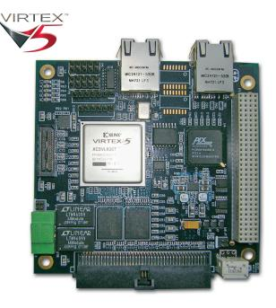
FreeForm/PCI-104 is a flexible reconfigurable board that combines a user programmable FPGA with a 32-Bit, 33MHz PCI-104 interface. The advantages of PCI-104's high bandwidth along with the versatile FPGA architecture allows users to create a high speed data interface and control solution that is uniquely suited to each individual application.
